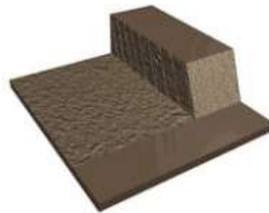
Fig. 3b. The shape of the working place after removal of the rock with using the inclinometer@system
