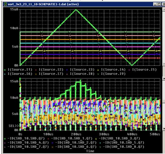
Fig. 6. Simulation results of sorting structure for  $V_{dd}=2.5V$ ,  $D_{max}=16\mu A$ ,  $T=18\mu s$  in the case of one ramp / falling signal and nine constant
