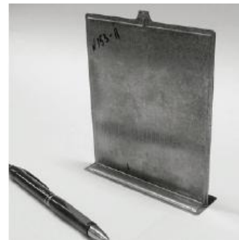
Figure 1-Design with integrated flat heat pipe
