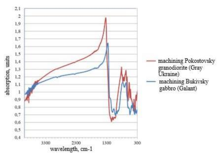
wavelength range to identify differences between these types stone and of to determine the natural processing stone efficiency. As can be seen from Fig. 1, Pokostivsky granodiorite (Gray Ukraine) and **Bukivsky** gabbro (Galant) have different infrared which is spectra, explained bv the
