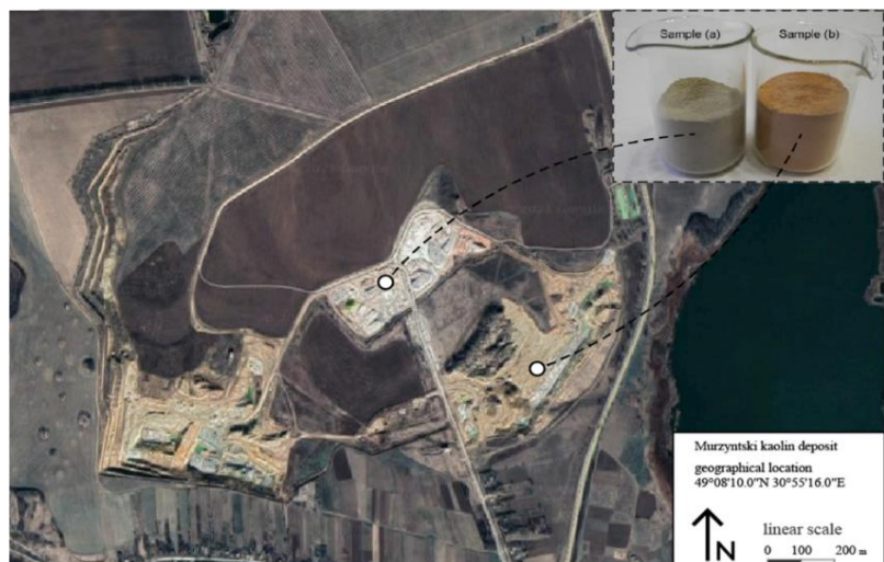
Figure 1. Kaolin samples from the Murzyntski deposit (a) white kaolin and (b) red kaolin
