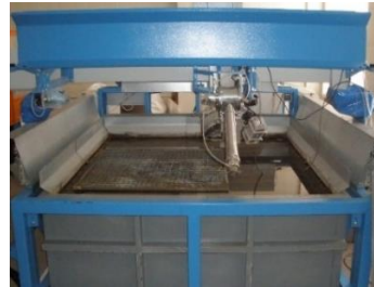
Figure 2 Current AWJM system and typical support structure configuration
